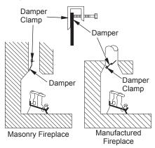
Figure 3 - Attaching Damper Clamp
